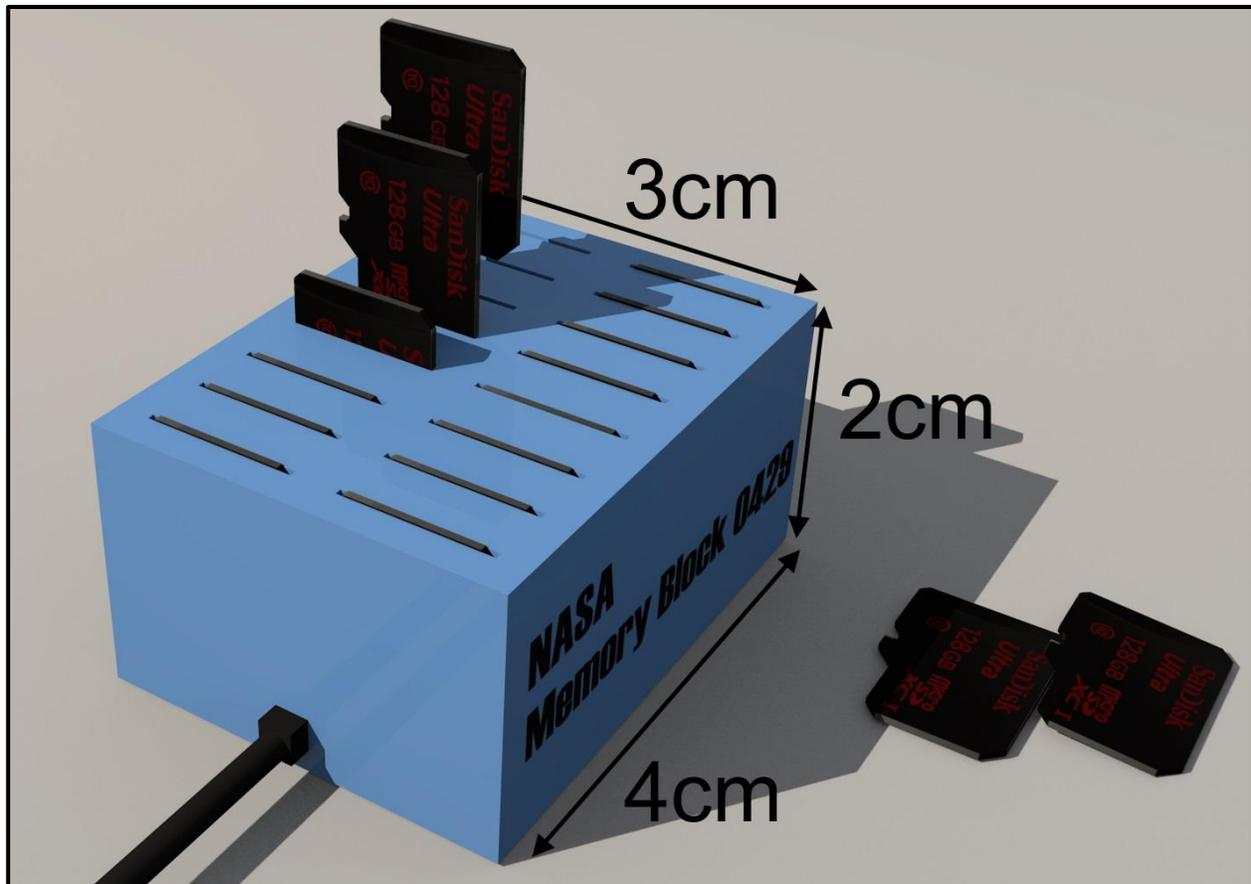
An interface box which houses 16 of these cards would be very light and very compact (as shown in the image above), yet have a capacity of 2 Terabytes (16 x 128GB), rising to 16 Terabytes as the technology improves. This would allow astronauts and re-supply missions to transport significant amounts of data to and from Mars.
