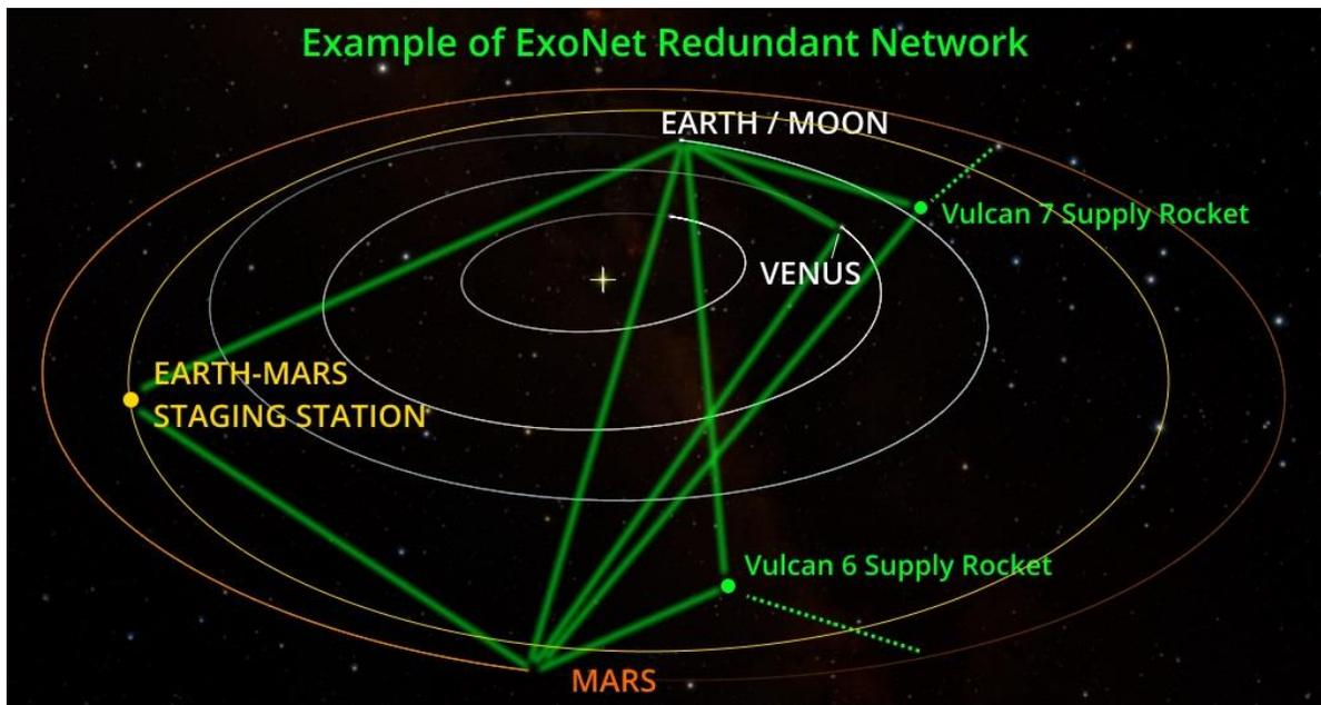
An algorithm on each site would calculate the shortest path for any message (based upon the current orbit position of each other site), but data would also be able to use alternative routes in event of a problem.
